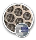
Our sintered wire mesh is available in standard configurations with up to 7 layers of media to meet the widest array of applications. The layers are compressed, sinter bonded and calendared to produce a uniform surface. Options include perforated plate or woven steel wire providing very high mechanical strength.
